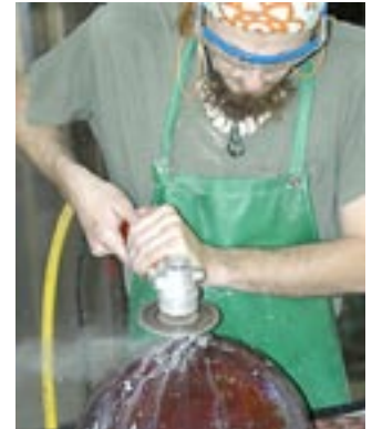
16. A small amount of shaping can be done with the grinder. The casting glass is softer than most other types of glass but still requires diamond abrasives to be efficiently
