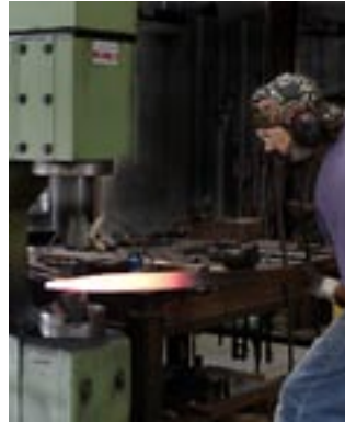
21. As the steel is hit about 220 times per minute with a radiused die, it stretches in length, becoming thinner in the areas that receive more blows. The steel may be reheated as necessary.
