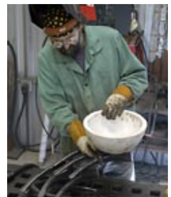
27. As the piece grows and assumes its identity practical considerations must be attended to. The interface between glass and steel is critical to achieve balance. A plaster cast of the generic hemisphere is used for fitting.
