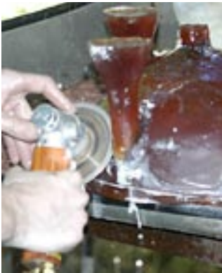
15. The sprues are cut from the casting using a water-fed diamond saw blade on a pneumatic angle grinder.
