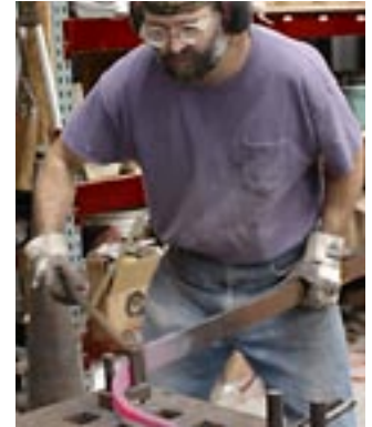
22. The hot part is then bent with bending forks to the desired curve. Once the steel has cooled it will be very difficult to bend the thick stock.
