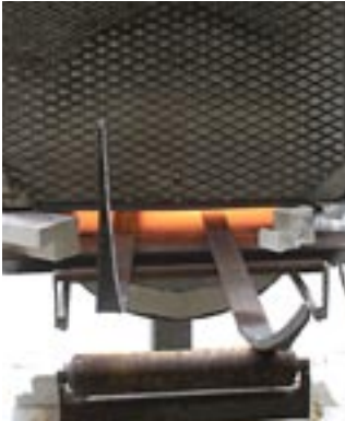
19. Rectangular bars of steel are heated to 2100°F in a gas-burning forge. Even when the end of the bar is glowing yellow hot it can still be handled by the unheated end.
