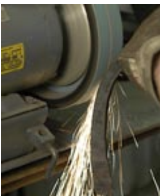
24. After being cut from the bar, the forged end has its edges sanded and ends rounded. The remainder of the bar will be reheated and another piece forged and cut off.
