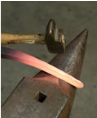
23. The curve and edges are refined using hammer and anvil. A combination of tradition and innovation work best to achieve the goals of the work: new forms that speak to contemporary aesthetics with timeless materials.
