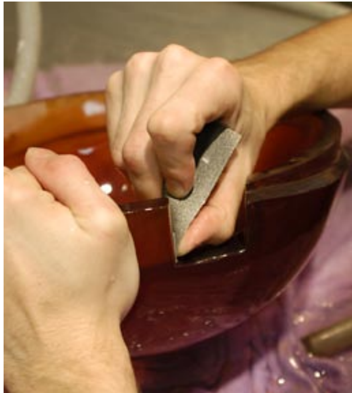
12. Demolding is the moment of truth, when it is revealed as to whether the work has turned out as planned. Extreme care must be taken not to damage the glass.
