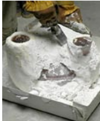
12. Demolding is the moment of truth, when it is revealed as to whether the work has turned out as planned. Extreme care must be taken not to damage the glass.
