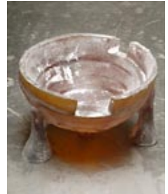
14. The demolded glass casting has a slightly rough surface. There are frequently spurs and fins which will have to be removed.
