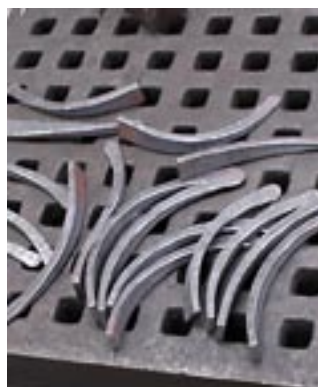
25. A pile of parts is produced, each unique in its details, but falling into a category of stock size, taper and curve dimensions.
