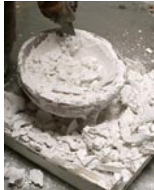
13. Demolding is akin to unearthing a fossil: incrementally the treasure is uncovered. The plaster investment can only be used one time.
